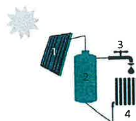
1: Zonnecollector | 2: Opslagvat zonneboiler | 3: Sanitair warm water 4: Radiator en verwarming 5: Tap water
